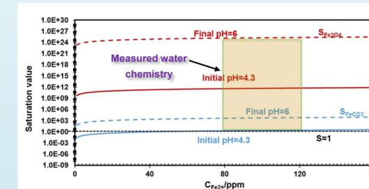
The absence of apparent corrosion product layer at a high saturation value suggested that the imidazoline-type inhibitor can also prevent the formation of corrosion product.
