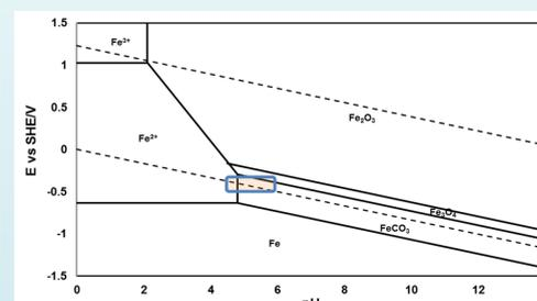
The corrosion product is likely a mixture of FeCO<sub>3</sub> and Fe<sub>3</sub>O<sub>4</sub> at the tested conditions: 150°C, 2 bar CO<sub>2</sub>.
